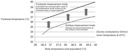
This unit measures the temperature at the surface of the forehead by sensing infrared emission of the skin at the measured point, and then calculates the oral-equivalent value using a unique algorithm (forehead measurement mode) based on actual body temperature survey data.
