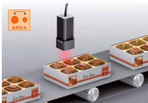
that users can understand and an easy intuitive method that saves time. The ZFV comes with a complete user interface, so a PC is unnecessary. The user interface consists of a crisp colour LCD screen and a few buttons. A simple menu guides you through the set-up procedure. To minimise installation effort, the sensor head comes with an integrated light with a field of view of up to 150 mm.
