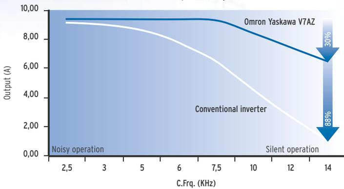
Conventional inverter vs V7 Amps Derating - 400 V-4,0 Kw at 50°C
