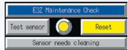
Example of a Smart Active Part for E3Z maintenance
