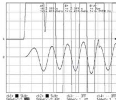
**Fig.3: Rigid load, with “tuning-less” function (Dynamic Self-Tuning)**
