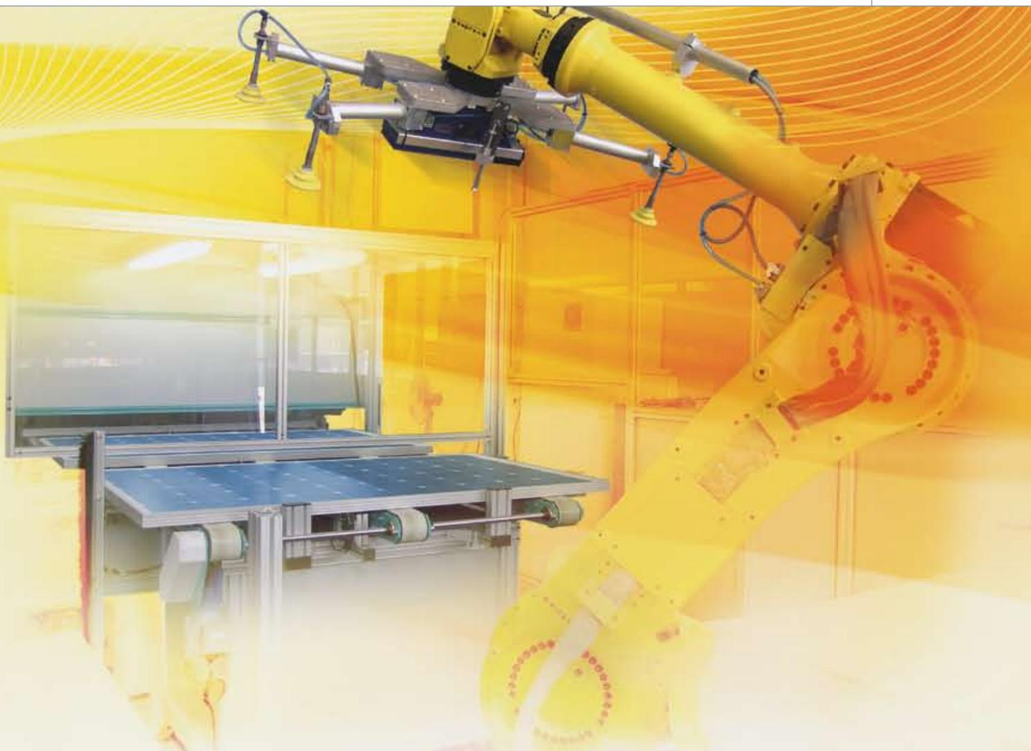
The safety system is controlled by an NE1A Safety Network Controller, which has expansion modules along the production line on a DeviceNet bus. This set-up controls the emergency stop pushbuttons at each of the robot stations, limit switches on the safety doors around the robots, and F3S-TGR-CL safety light curtains protecting the loading/unloading sections.
