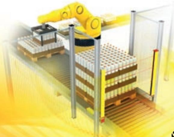
Extended muting functions - infinite muting for applications where the material is blocking access to the dangerous zone and where process time is long. Typical applications are conveyor systems in the ceramics or beverage industries.
