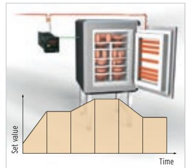
In time-based process applications, banks are used to hold PID and alarm values. They can also hold soak times as another way of creating an SV program.
