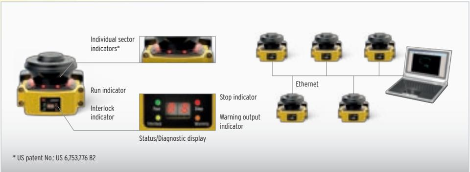
Simple monitoring of several OS32C units is achieved by integrated Ethernet communication for programming and maintenance. Clear maintenance information is given by sector indicators for easy recognition of which sector is blocked and the OS32C's status is given by a 7-segment display.
