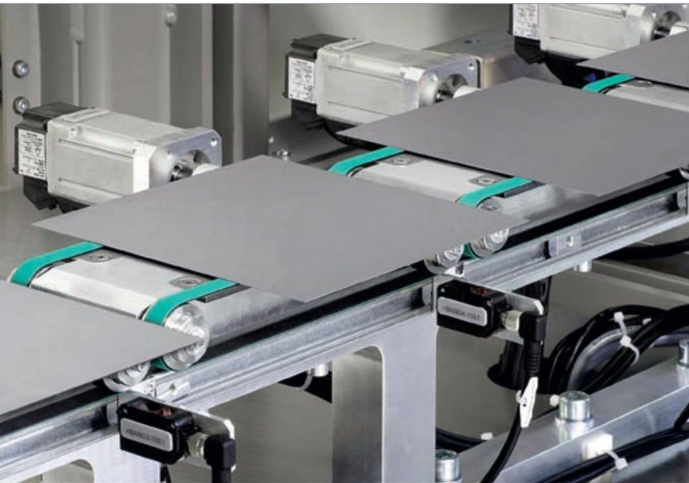
*Wafer conveyor controlled by G5 servo motors with EtherCAT motion bus and optical E3Z family sensor*
