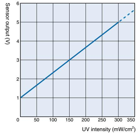
F3UV-XA + F3UV-HM + F32-300 (output characteristics at 300 mW/cm<sup>2</sup> when sensitivity is set)
