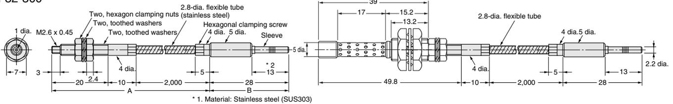
Note: Heat resistance temperature is 300°C for part A and 110°C for part B (part inserted in unit). However, take care that parts inserted in unit (parts marked are within operating temperature range of amplifier.
