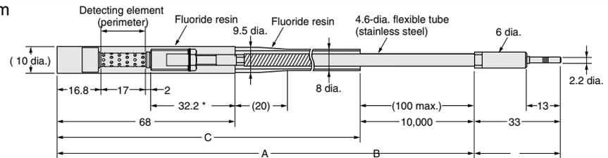
Note 1. Heat resistance temperature is 150°C for part A and 110°C for part B (part inserted in unit).
