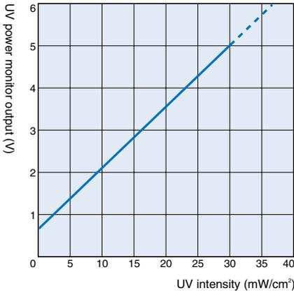
F3UV-A03 (output characteristics when output at 3 mW/cm<sup>2</sup> is set to 5 V)
