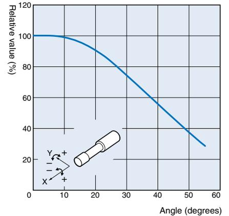
Note: X-direction output fluctuation is ±10% F.S. or less through 360° revolution
