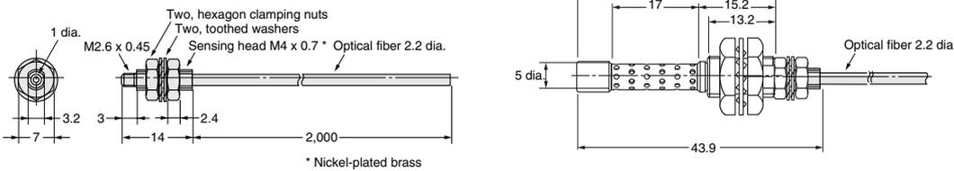
Note: indicates that free-cutting is possible. Free-cutting is not possible on units that are not marked with .
