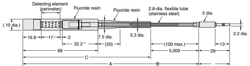
Note 1. Heat resistance temperature is 150°C for part A and 110°C for part B (part inserted in unit).
