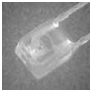
High output pin-point light source LED (wave length: 670 nm)
