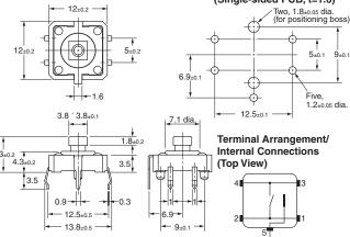
Note: The numbers used for terminals in the following graphics are indicated in the "Bottom View" diagram below. In this diagram, the Switch is rotated so that the terminals are on the right and left-hand sides, and the OMRON logo appears the right way up.
