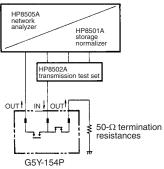
The following characteristics are measured with contacts unrelated to the measurement terminated at  $50\Omega$ , when a signal is applied from input terminal 11 to output terminal 8 or from input terminal 11 to output terminal 11 to output terminal 18 or from input terminal 19 of the sample.
