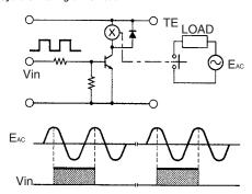
If the relay operates in synchronization with the supply voltage, the life of the relay may be shortened. When designing the control system in which the relay is used, estimate the life of the relay and thus the reliability of the overall system under actual operating conditions. Moreover, construct the circuit so that the relay operates in a random phase or in the vicinity of the zero point.
