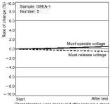
Characteristics were measured after applying a shock of 490 m<sup>2</sup>/s to the test piece 3 times each in 6 directions along 3 axes. The percentage rate of change is the average value for all of the samples.
