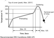
Note: Do not submerge the relay in a solder bath. Doing so will deform the resin causing faulty operation.
