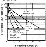
However, with a DC load, it may become difficult to break the circuit of 48 V or more due to arcing. Determine the suitability of the relay in actual usage testing.
