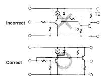
A circuit that produces a control output as soon as the relay operates must be carefully designed. In the example on the left, electrode dark current flows as shown when the relay operates. When dark current flows into the relay coil, the relay's resistivity to shock and vibration may degrade.
