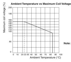
Note: The maximum coil voltage refers to the maximum value in a varying range of operating power voltage, not a continuous voltage.
