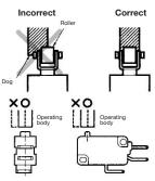
Make sure that the operating body moves in a direction where the actuator moves. If the actuator is a pin plunger type, make sure that the operating body presses the pin plunger vertically.
