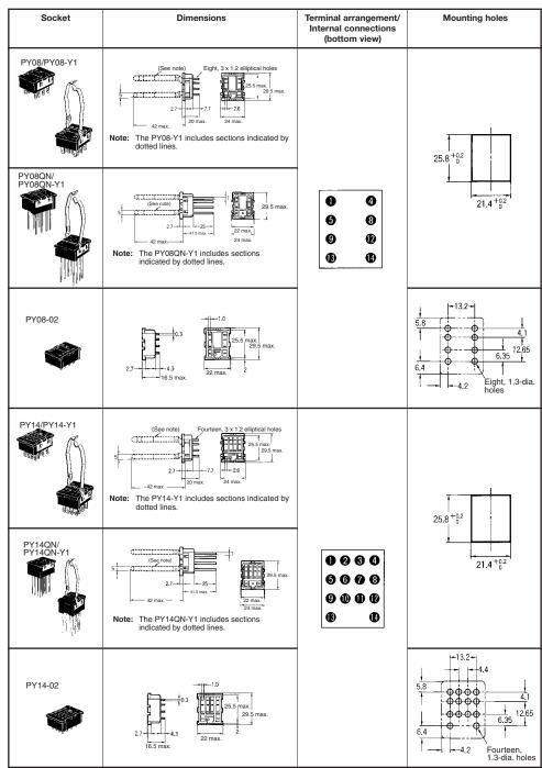
Note: Use a panel with plate thickness of 1 to 2 mm for mounting the Sockets.
