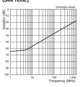
High-frequency Characteristics (Insertion Loss) (See note.)
