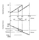
Make sure that operating body returns the actuator to the free position when the operating body has moved if the Switch is used to form a normally closed (NC) circuit. If the Switch is used to forma normally open (NO) circuit, the operating body must move the Switch actuator to a distance of 70% to 100% of the rated overtravel (OT) of the Switch.
