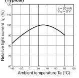
Dark Current vs. Ambient Temperature Characteristics (Typical)
