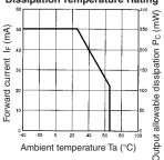
LED Current vs. Ambient Temperature Characteristics (Typical)
