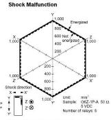
Conditions: Shock is applied in TX, TY, and TZ directions three times each with and without energizing the Relays to check for contact malfunctions.
