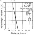
Sensing Position Characteristics (EE-SV3-C(S))
