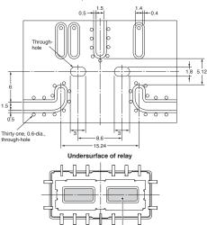
Note: To obtain high-frequency characteristics close to the charts shown on page ?, solder the convex point on the undersurface of the relay to the ground pattern of the substrate.
