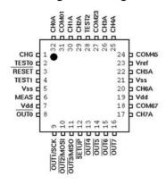
Note 1: Pins TEST0 - 2 are used for testing during manufacture of the IC.
