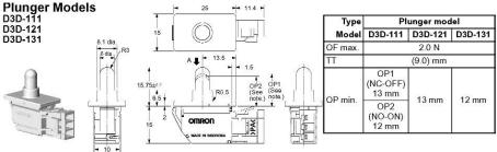
Note: The dimensions OP1 and OP2 apply to the D3D-111 only. The D3D-121 and D3D-131 are SPST-NC and SPST-NO respectively and so therefore have only one corresponding dimension here (OP).
