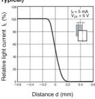
EE-SX1109 Sensing Position Characteristics (Typical)
