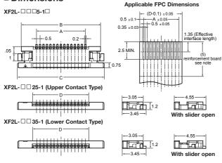
Note 1: Use polyimide and thermoset adhesive for reinforcement film material.
