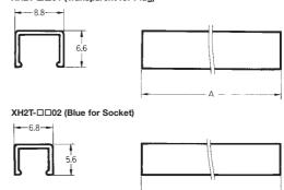
Attach these Dust Covers to Connectors that are not in use. They do not protect the Connectors from flux during automated soldering.
