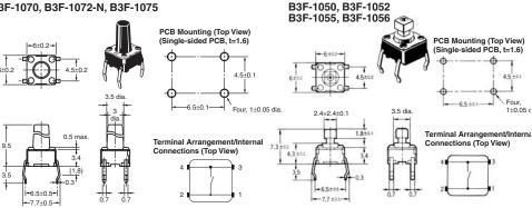
Horizontal, Projected Plunger Type (with Ground Terminal)
