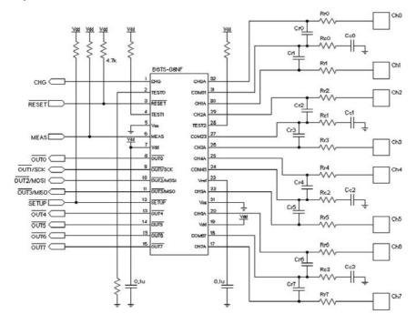
Note 1: Connect Rr, Cr, Rc, and Cc to each touch electrode, as shown in the above figure.
