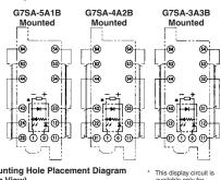
**Mounting Hole Placement Diagram** (Top View)
