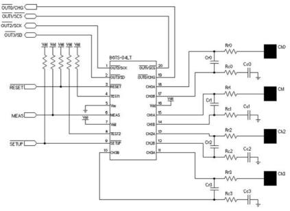
Note 1: Connect Rr, Cr, Rc, and Cc to each touch electrode, as shown in the above figure.
