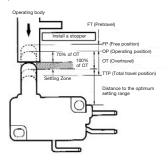
If the stroke is set in the vicinity of the operating position (OP) or at the releasing position (RP), switching operation may become unstable. As a result, the Switch cannot ensure high reliability. Furthermore, the Switch may malfunction due to vibration or shock. If the stroke is at the total travel position (TTP), the momentary inertia of the operating body may damage the actuator or the Switch itself. Furthermore, the life of the Switch may be shortened.
