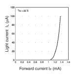
**Light Current vs. Forward Current** Characteristics (Typical)
