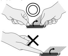
Do not engage the slider (lever) past its primary location during the unlocking process. Doing so may result in damage to the connector or contact failure.
