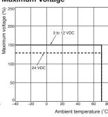
Note: "Maximum voltage" is the maximum voltage that can be applied to the Relay coil.
