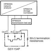
The following characteristics are measured with contacts unrelated to the measurement terminated at  $50\Omega$ , when a signal is applied from input terminal 11 to output terminal 8 or from input terminal 11 to output terminal 11 to output terminal 8.
