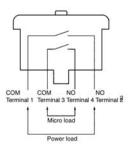
**Note:** The circuit switching power loads has a snap-action mechanism and the circuit switching micro loads has a slow-action mechanism.
