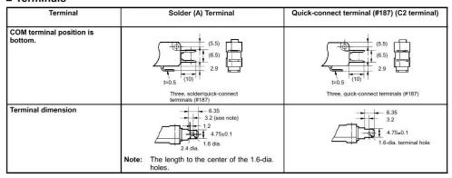
Note: The above is for the SPDT contact specifications.
