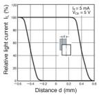
EE-SX1107/1108/1109/1131 Sensing Position Characteristics (Typical)
