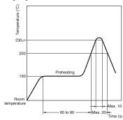
Note: The above heating curve applies if the PCB thickness is 1.6 mm
