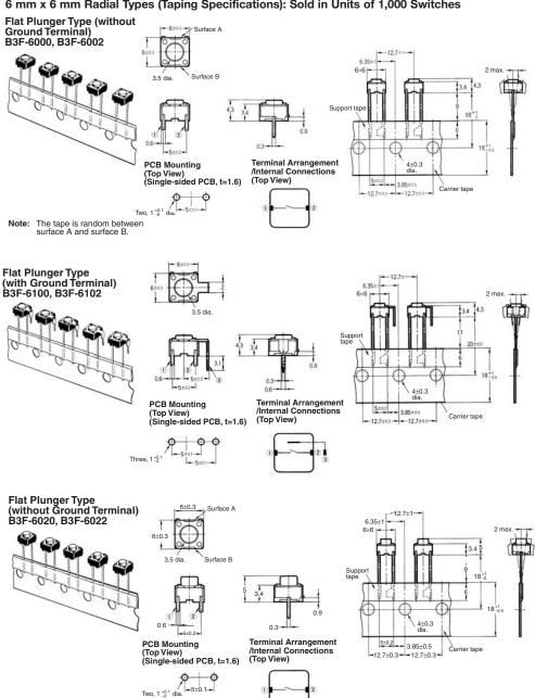
Note: The tape is random between surface A and surface B.
