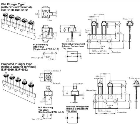
Note: The tape is random between surface A and surface B.
