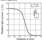
EE-SX1131 Sensing Position Characteristics (Typical)
