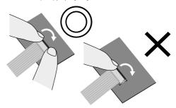
Do not apply horizontally to the PCB, when locking the slider (lever). Doing so may result in damage to the connector or contact failure.
