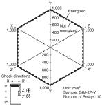
Conditions: Shock is applied in ±x, ±y, ±z directions three times each with and without energizing the relays to check the number of contact malfunctions.
