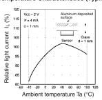
Dark Current vs. Ambient Temperature Characteristics (Typical)
