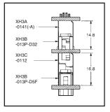
Fine-fit Backplane Connector and Fine-fit Short Terminal Connector Combinations
