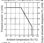
LED Current vs. Ambient Temperature Characteristics (Typical)
