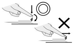
When unlocking the slider (lever), place your fingers on either side or the whole of the slider (lever) and slowly lift the slider (lever) up and away.
