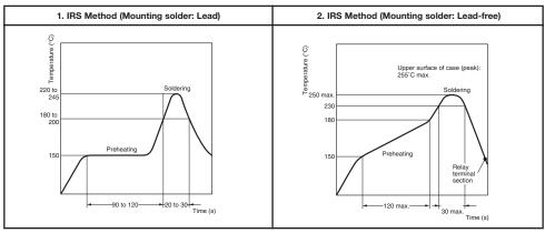
Note: Do not submerge the relay in a solder bath. Doing so will deform the resin causing faulty operation.
