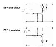
When the transistor is used in a emitter-follower configuration (i.e., the collector is grounded), give adequate consideration to the voltage across the collector and emitter. The required voltage must be applied to the relay.
