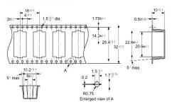
Note: The radius of the unmarked corner is 0.3 mm.
