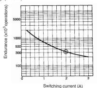
However, with a DC load, it may become difficult to break a circuit of 48 V or more, due to arcing. Determine suitability of the Relay in actual usage testing. Correlation between the contact ratings is as shown below.
