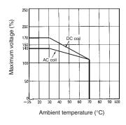
**Note:** The maximum voltage refers to the maximum value in a varying range of operating power voltage, not a continuous voltage.
