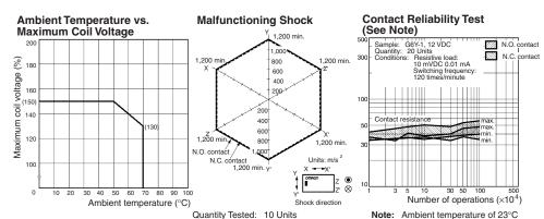
Note: The maximum coil voltage refers to the maximum value in a varying range of operating power voltage, not a continuous voltage. Test Method: Shock was applied 3 times in each direction with and with out excitation and the level a which the shock caused male
