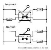
Even in a "correct" circuit, note that the insulation performance of the switch may deteriorate and the switch life may be shortened because one load is connected to one contact.
