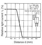
Sensing Position Characteristics (EE-SH3-C(S))
