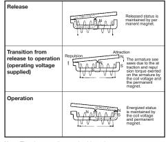
Note: The above applies to a latching relay.
