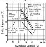
The life expectancy of the relay can be determined from the "Endurance" curve shown below, based on the rated switching current (I<sub>1</sub>) obtained above. For instance, the electrical endurance at the obtained maximum switching current of 2 A is slightly over 300,000 operations (see circled point on graph below).
