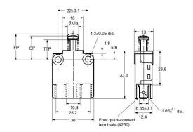
Note: NC-OFF: The force applied to the actuator to cause it to move from the free position to the position at which the NC contact opens.
