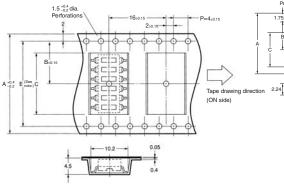
**Note:** The perforations along both sides are for 8-pole Switches only. The perforations on the bottom of the diagram are not for 4- and 6-pole Switches.
