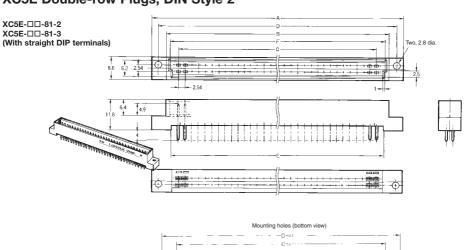
Note: Dimensions are given for XC5E----81-2. The dimension and shape of the XC5E----81-3 are different contact OMRON for further information.
