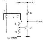
Figure 16. Equivalent Circuit
