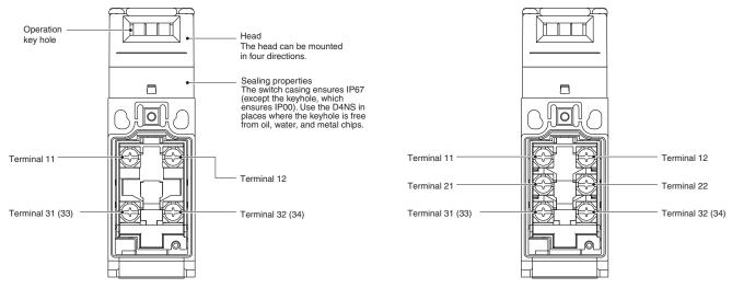
Note: The 2-conduit models have the same terminal arrangement.
