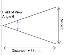
Note: The Recess value of 33 mm is the distance from the reader front face to the image sensor inside the reader. The Distance and Recess values are added together for the FOV Scan Area calculation.
