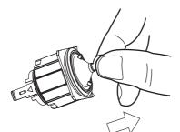
2) After you remove the cap, you can remove the legend plunger and engrave it.
