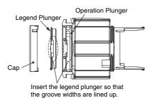
2) Attach the cap, aligning the slots on the slot on the cap with the tab on the operation plunger.
