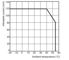
**Note:** The value for standard mounting. Note that the derating curve differs depending on the mounting.
