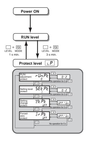
The "key protect" function limits level and parameter changes using key operations. There are 4 kinds of key protection. The parameters, settings, and details of each kind of protection are outlined below.
