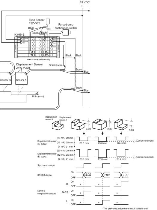
\* The previous judgement result is held until the Sync Sensor turns ON. (All outputs turn OFF when RESET input is received.)
