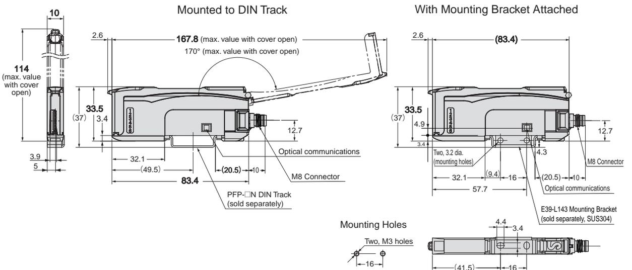
**Amplifier Unit with Connector for Sensor Communications Unit**
