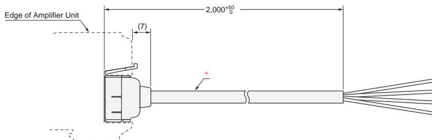
\*4-dia. cable with 4 conductors, Standard cable length: 2 m (Conductor cross-section: 0.2 mm<sup>2</sup> (AWG24), Insulation diameter: 1.1 mm)
