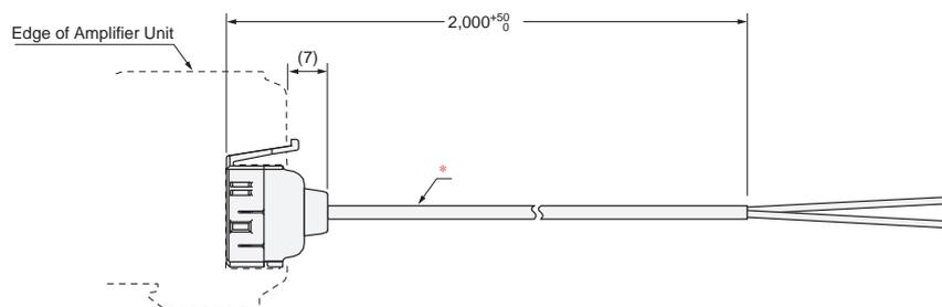
\*4-dia. cable with 2 conductors, Standard cable length: 2 m (Conductor cross-section: 0.2 mm<sup>2</sup> (AWG24), Insulation diameter: 1.1 mm)
