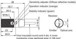
Vinyl insurated round cord 4 dia. 4 cores (conductor cross sectional area: 0.128 mm² (AWG26)/insulation outside diameter: 0.85 dia.) standard length 2 m
