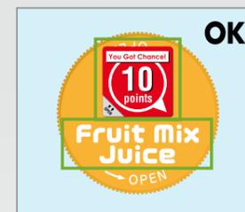
The correct position of workpieces with an inconsistent orientation can be measured through automatic detection of the offset of the workpiece in relation to a registered standard model.
