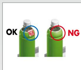
This is a standard search inspection item. This type of search is used to detect items like labels, identify shapes, or positions.
