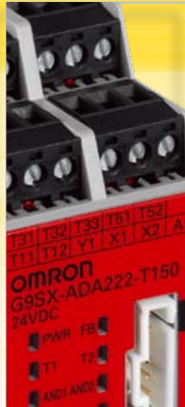
Terminals can be either screw-type or screw-less spring-type.
