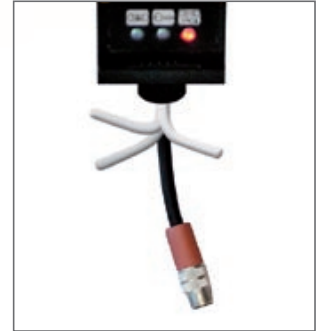
Connection via M12 cable/plug.
