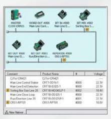
Omron's CX-One software has a special screen that displays maintenance information without any need for programming. It also lets you make and change settings with ease (e.g. alarms).
