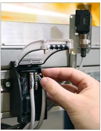
Simply push in the terminated I/O wiring. Close the cover and you're done.
