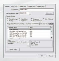
Smart Analogue I/O performs data preprocessing to help you reduce PLC programming. It can handle scaling, alarms, totalizing and even rate-ofchange calculations. Just tick the boxes and set the parameters.
