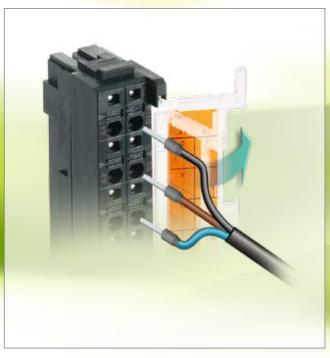
No need to stop: The reliable 3-piece construction enables you to swap modules during operation, without rewiring. After you have set up all units, their parameters can be backed up in the bus interface unit at the flick of a switch. Restoring the settings is even simpler; after hot-swapping a unit, all settings are automatically loaded.
