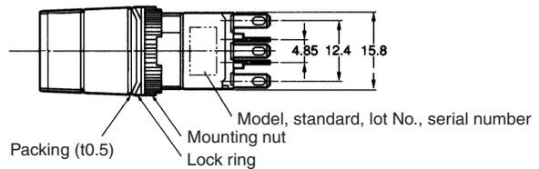
The following diagrams show the rectangular model as a representative example. The lamp terminal is also provided with non-lighted models.
