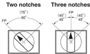
Note: 1. The angle used for automatic reset is shown in parentheses.
