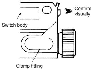
If the clamp is properly inserted up to the full depth, it will not slide out easily. Be sure to carefully confirm all the above items.
