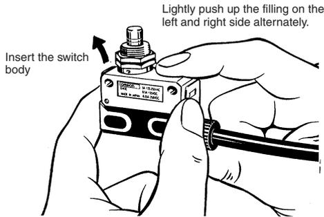
Be sure that the clamp is inserted to the full depth, because the Switch will not function properly if one of the clamps is improperly inserted.
