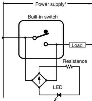
**Note:** \*An external 24VDC power supply can be used, eg. OMRON S8VS.
