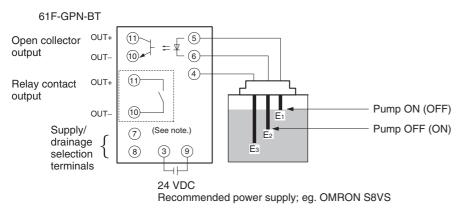
Note: The part within the dotted-line box is for the 61F-GPN-BC (relay-output type) only.
