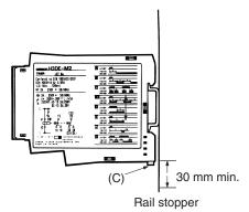
The H3DE can be mounted and dismounted with ease if a distance of 30 mm or more is kept between the H3DE and the top surface of other equipment located below the H3DE.
