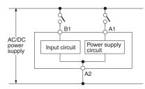
Since the input circuit and the power supply circuit are configured independently, the input circuit can be turned on or off irrespective of the on/off state of the power supply.
