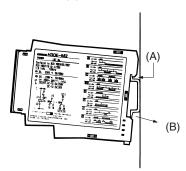
When dismounting the H3DE, pull out portion (C) with a flat-blade screwdriver and remove the Timer from the mounting DIN-rail.
