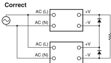
**Note: 1.** The diode is connected as shown in the figure. If the load is short-circuited, a reverse voltage will be generated inside the Power Supply. If this occurs the Power Supply may possibly deteriorate or be damaged. Always connect a diode as shown in the figure.
