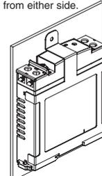
Note: The Side-mounting Bracket can be mounted from either side.
