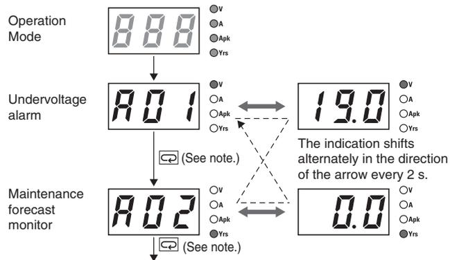
**Note:** 1. When undervoltage alarm is indicated: Press → output load indication When the maintenance forecast monitor or overheat alarm is indicated: Press → undervoltage alarm indication
