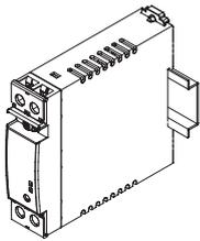
Horizontal mounting with DIN-rail
