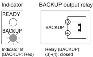
When the backup operation functions, the energy in the internal capacitor will be discharged to the load. When the voltage of the power supply then recovers, the S8T-DCBU-02 will start charging the capacitor. Up to 60 seconds is required to charge the capacitor completely. The backup operation may therefore not function for the required period if the backup operation starts while the capacitor is being charged.
