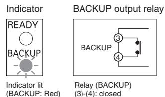
**Note:** Check the backup operation under conditions that are safe and will cause no problems if the backup operation fails.
