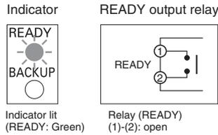
The following status will occur if there is an error in the charge voltage of the internal capacitor or the output voltage of the S8T-DCBU-02.
