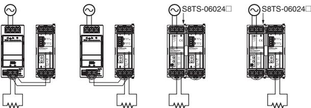
**Note:** Use the largest wire size possible and keep the wiring distance as short as possible. If the voltage drop caused by the wiring material is too large, the backup operation may not be sufficient.
