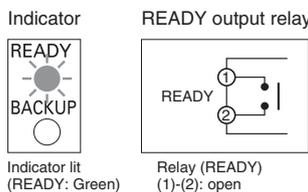
**Note:** Up to 60 seconds is required to charge the internal capacitor before the indicator lights.
