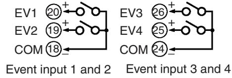
Terminals 18 and 24 (COM) are connected internally.
