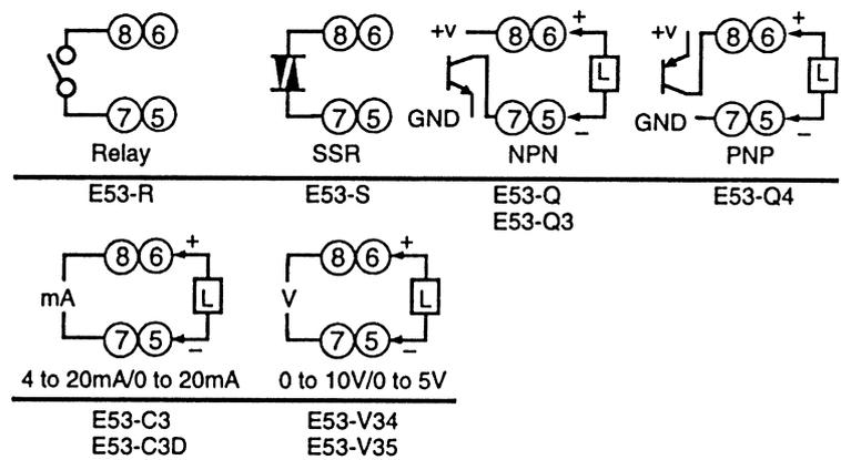
With E53-V□□ Output Units, approx. 2 V is output for one second after the power is interrupted.
