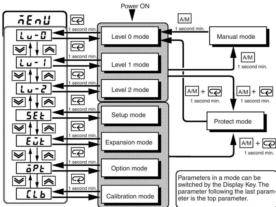
**Note:** The control of the Digital Controller is reset when the Digital Controller is in setup, expansion, option, or calibration mode, in which case the control and auxiliary outputs are OFF. The reset condition will be canceled when the Digital Controller is in any mode other than the above.
