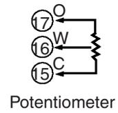
For details on CT inputs, refer to *Appendix, About Current Transformer* in the *E5AK/E5EK User's Manual (H83/H85)*. For details on the potentiometer, refer to the *Instruction Manual* for the valve connected to the Controller. The variable resistance range is 100 Ω to 2.5 kΩ
