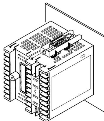
3. Tighten the mounting bracket screws on the upper and lower parts of the E5AK in small increments alternately and equally until the ratchet start to slide.
