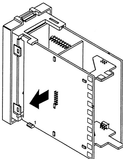
2. Insert the Option Unit into the socket for option 1. The following diagram shows the relationship between the Option Unit and mounting position.
