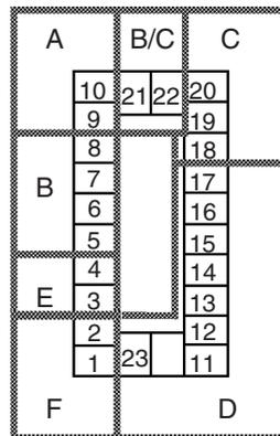
**Note:** Terminals 21 and 22 of the E5EK belong to the B block when a transfer output is set to option 1 and to the C block for other Option Units.
