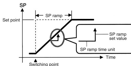
The change rate during the SP ramp is specified by the "SP ramp set value" and "SP ramp time unit" parameters. At the "SP ramp set value" default "0," the SP ramp function is disabled.
